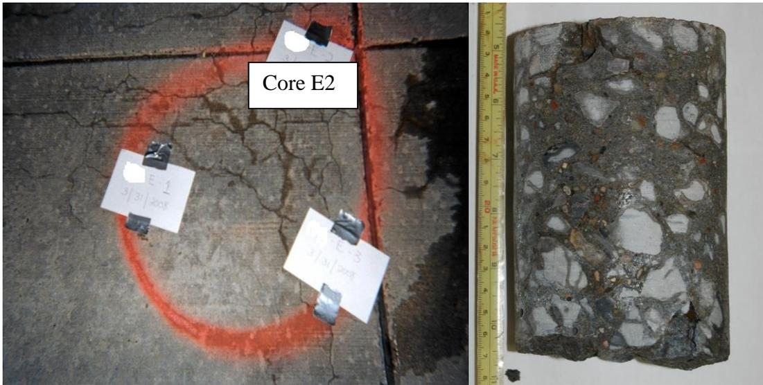
(A) Photograph of core and its location (Echo-2) showing cracks near the surface
