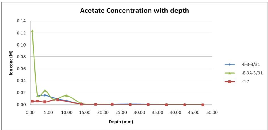
Figure 16 – Profile of acetate ions in Taxiway Echo cores. Note that the Y-axis scale is not the same in all the graphs
