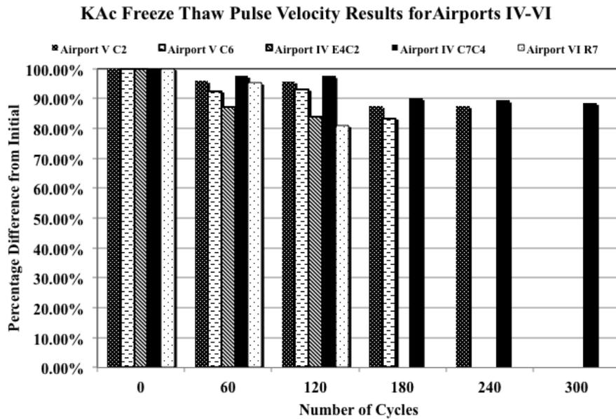
Figure 18 – 6.4M KAc Freeze Thaw Pulse Velocity Results for Airports IV-VI
