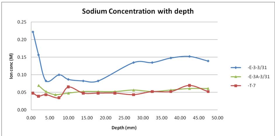
Figure 12 – Profile of sodium ions in Taxiway Echo cores.
