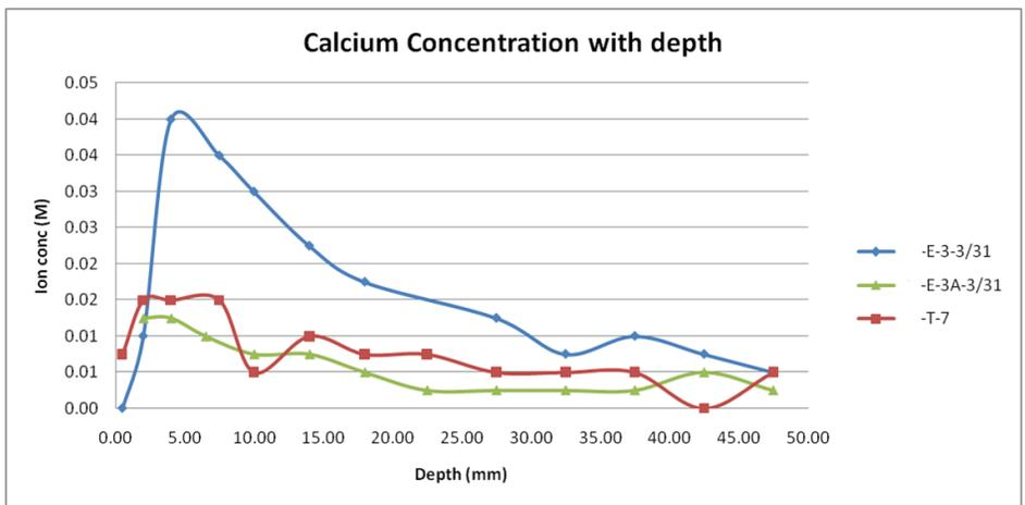
Figure 13 – Profile of calcium ions in Taxiway Echo cores. Note that the Y-axis scale is not the same in all the graphs
