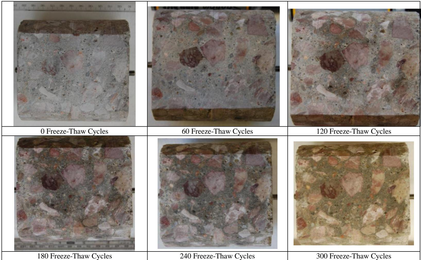
Figure 19 – Visual Condition of Airport IV Taxiway Echo 4 Core 2 (exposed to deionized water) During the Freeze Thaw Testing
