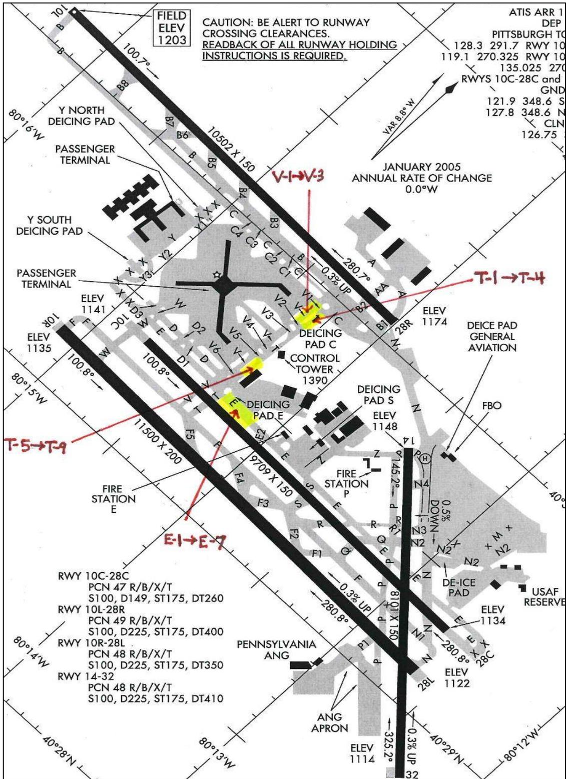
Figure 3 – Locations of distressed pavements and coring sites at Airport I.
