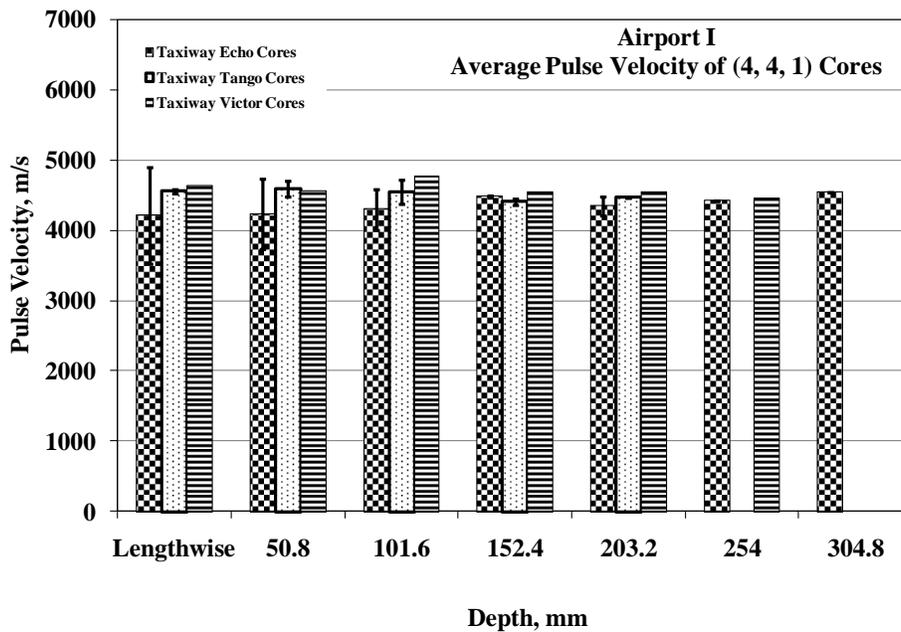
Figure 6 – Pulse velocity results from Airport I cores. The depth represents the distance from the surface of the pavement at which readings were taken on the cores.
