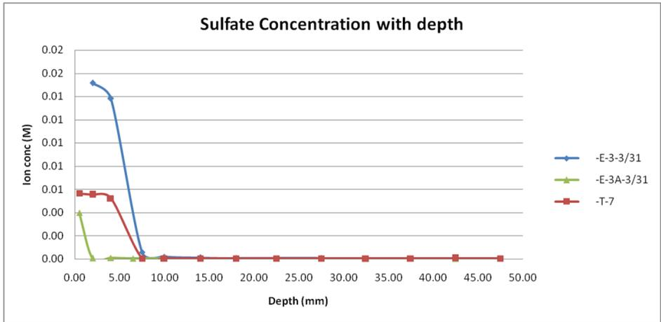
Figure 14 – Profile of sulfate ions in Taxiway Echo cores.
