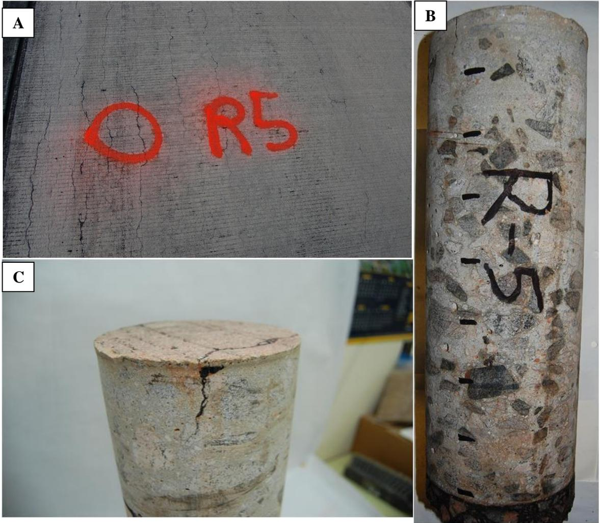
Figure 5B – (A) Typical location for coring in a distressed pavement (Runway at Airport VI) (B) – Physical condition of the core (C) The 5.75 in. diameter core was 16.38 inches long with a single crack running down from the pavement surface to about a depth of 2.5 inches.
