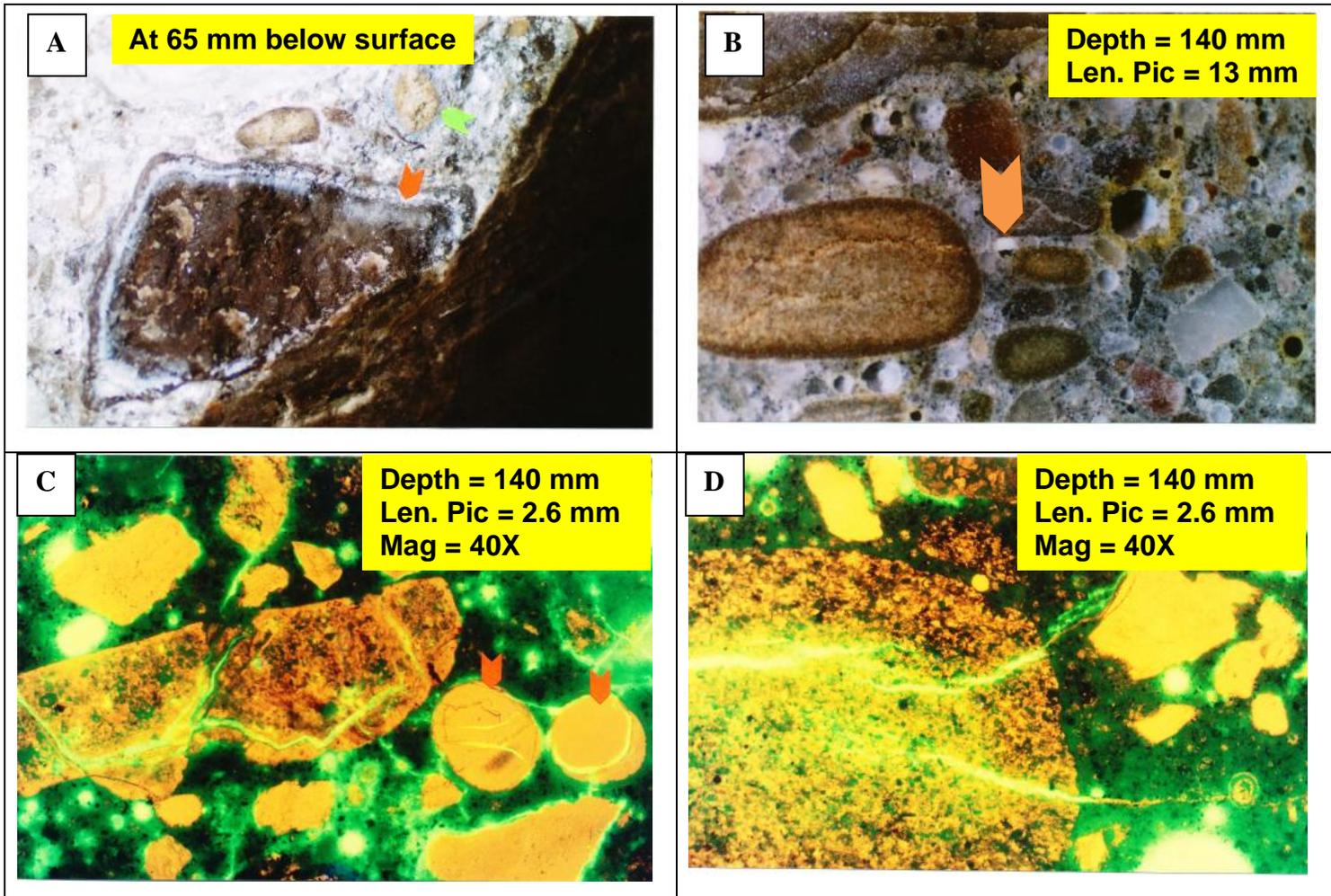
Figure 8 – Evidence of reacted aggregates and ASR gel at different depths in the core. Images A and B were taken using a stereo microscope on fractured and lapped specimens, respectively. Images C and D show thin sections subjected to transmitted polarized light and simultaneous reflected UV light. The orange arrows indicate ASR gel deposits.
