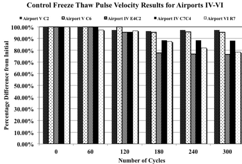
Figure 17 – Control Freeze Thaw Pulse Velocity Results for Airports IV-VI
