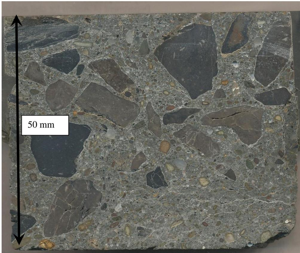
(B) Photograph of polished section from core Echo-5 from nearby location. The width of this specimen is 50 mm.
