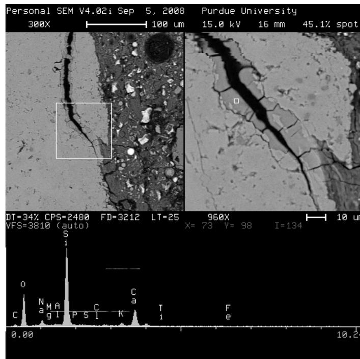
Figure 10B – Crack in aggregate filled with gel (with smaller cracks oriented perpendicular to the larger crack). Textural differences in matrix close to crack opening (right picture, bottom right corner).
