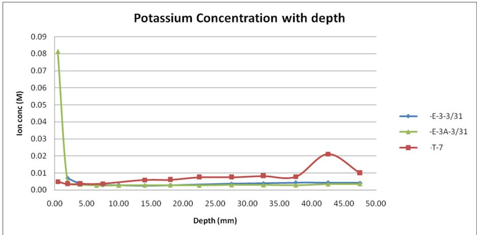
Figure 11 – Profile of potassium ions in Taxiway Echo cores.
