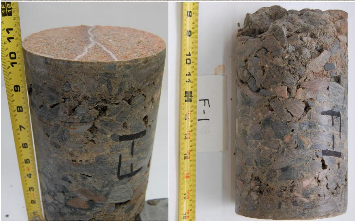
Figure 5C – (A) Typical location for coring in a distressed pavement (Taxiway Foxtrot at Airport VI) (B) – Physical condition of the core with significant honeycombing in the top 4 inches and from 7 - 12 inches below the pavement surface. The core was retrieved in two pieces, with 5.75 in. in diameter and a total length of 16.13 inches.
