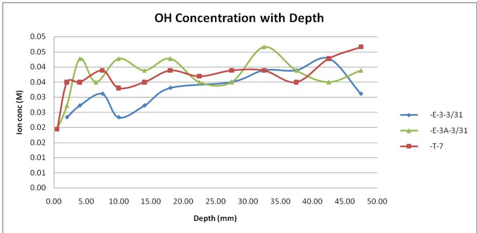
Figure 15 – Profile of hydroxyl ions in Taxiway Echo cores.
