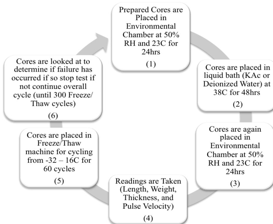
Figure 2 –Modified ASTM C 666 procedure to evaluate effect of KAc deicer exposure on freeze-thaw durability of concrete
