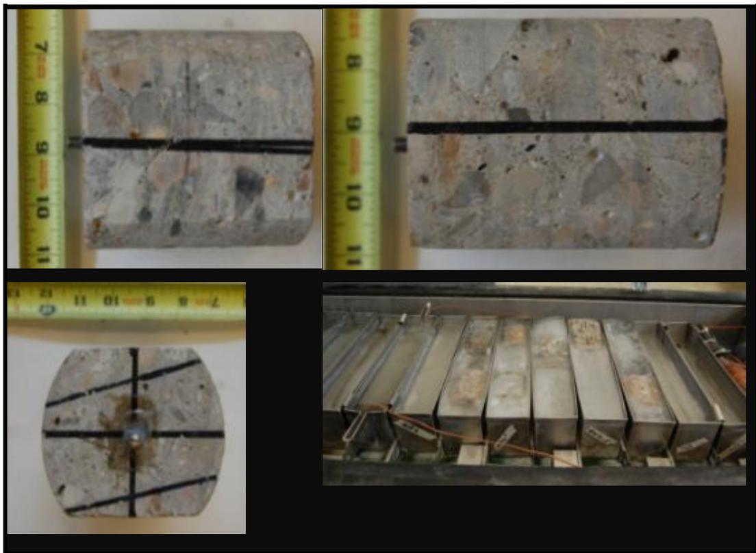
Figure 4 – Prepared Freeze Thaw Samples and Test Setup
