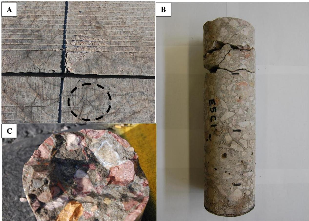
Figure 5A – (A) Typical location for coring in a distressed pavement (Taxiway Echo Connector 5 at Airport IV) (B) – Physical condition of the core showing cracks running down from the pavement surface (C) Fractured surface showing reaction rims and white reaction product surrounding coarse aggregate particles. The 3.75 in. diameter core is 15.50 inches long with multiple fractures in the core in the top 5 inches.
