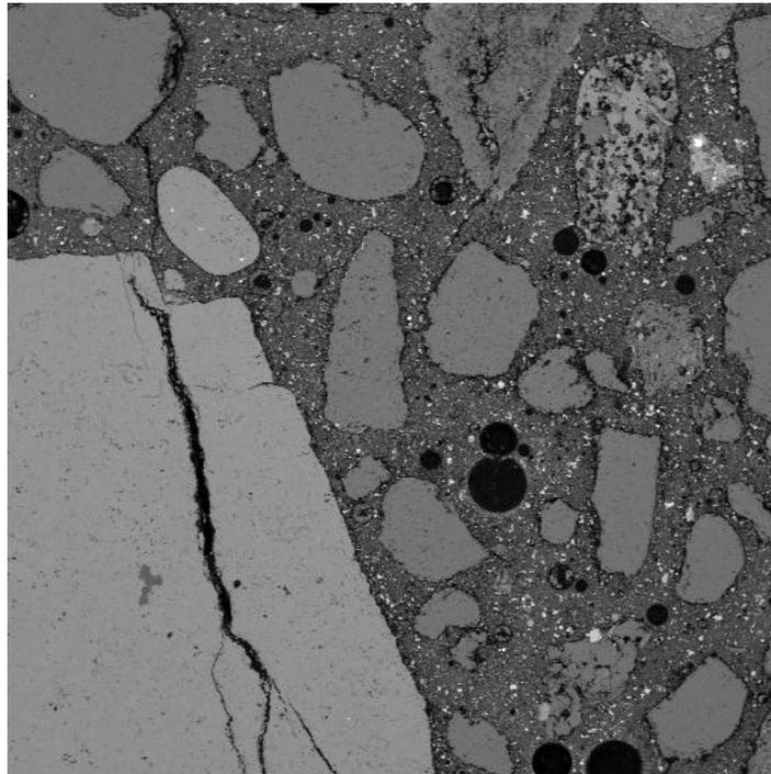
Figure 10A – Cracking in carbonate aggregate (at 30x magnification)
